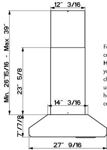
For higher ceilings an high ceiling kit (Part Number HIGHFORTIS) is available, see your dealer for information. The chimney extension replaces the upper chimney shipped with the hood and adds 21" to overall ceiling heights.
