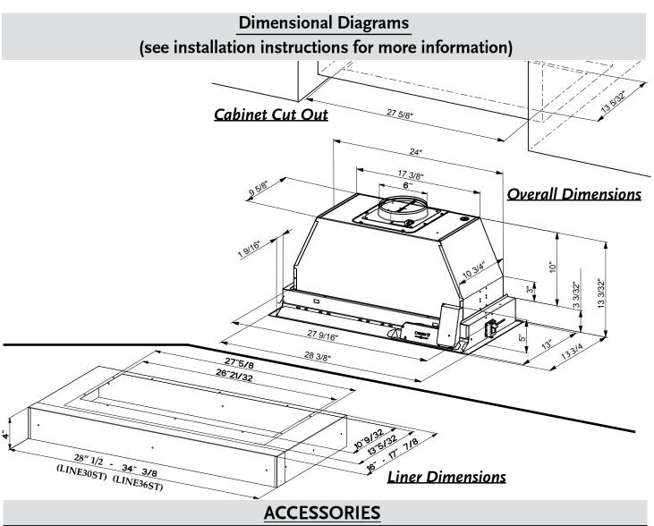
Stainless LinersSizeModel #Create a perfectly-sealed, non-combustible 4" tall<br/>perimeter to "line" the wood below the Inca HC. Depth<br/>adjustable from 16" - 17 7/8".30" SS Liner# LINE30ST
