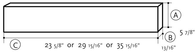
\* If you wish to keep the frame of the front panel and only replace the glass panel, the dimensions are as follows:  $A=5 \, 11/16$ ", B=1/8",  $C=23 \, 6/16$ " (for 24" model) or 29 11/16" (for 30" model) or 35 11/16" (for 36" model). The glass panel is 1/8" thick, but the frame is adjustable to accommodate a thinner panel like stainless steel.
