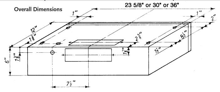
Custom Front Panel Dimensions - for replacing the entire front panel \*
