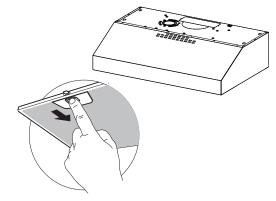
2 Remove the wiring box cover by unscrewing the 2 screws.
