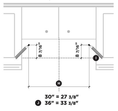
**3** Mark the wall for lower anchors. Mark 1" below the Step 2. Upper Anchors. Take care to keep level.
