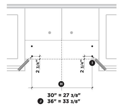
Drill a 3/16th hole directly into the wall at the center points marked in step 3. If fastener locations do not align with the studs, insert the purchased wall plugs in the holes.
