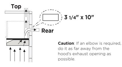
1 Choose the rectangular upper air outlet or rectangular rear air outlet and cut where indicated.(See page 18 for Rear Outlet)
