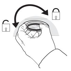
2 Replace the bulb with a new one of the same type, making sure that you insert the two pins properly into the housings on the lamp holder and twist to lock back in place.
