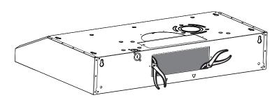
Install the included rectangular air outlet with two screws 🕞
