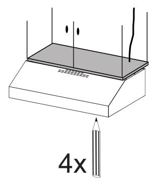
4 Attach the Hood body with 4 screws 🕒 from the bottom available with the hood.
