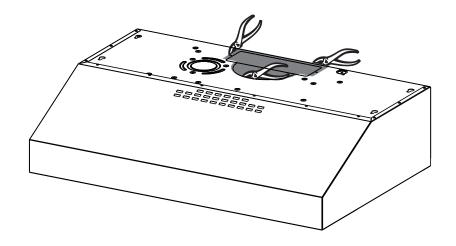
Install the Flange with Flange transition screws **F**. 2
