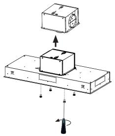
Attach the Flange 3 to the hood in the same location as the original motor box with the screws A provided in the hardware bag as shown
