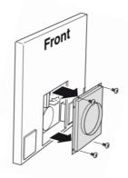
Attach the Flange 3 to the hood in the same location as the blocker plate using the screws A and B provided in the hardware bag.
